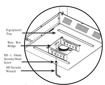
**Step 4.** Insert four (4) M5 x 10mm security screws and tighten using the M5 security wrench.
